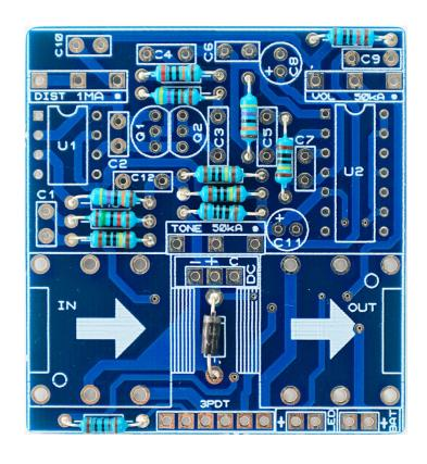
Place the resistors and diodes. If you have troubles reading the values, check out our "Reading Part Values" tutorial.
